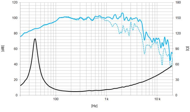
Note: Frequency response measured with loudspeaker standing on infinite baffle in anechoic chamber, 1W @ 1m Frequency response on axis Frequency response 45° off axis
