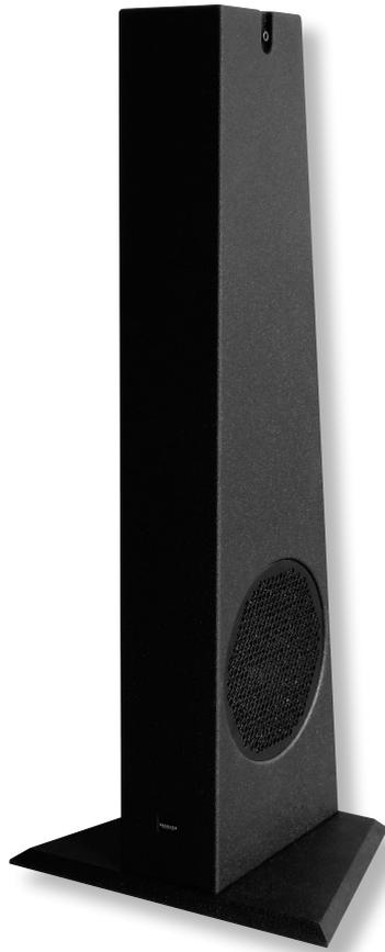
The GL Sub dp is a dedicated Subwoofer for the GL 16 System. With 140 cm height it enables the optimal positioning of a GL 16 for a sitting or standing audience. The 12" speaker is powered by a 1000 Watt amplifier with DSP. The GL Sub dp is especially suited for applications which require a unobtrusively looking GL 16 System with Subwoofer.
